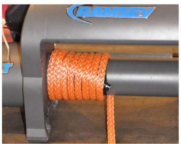
Always retain a minimum of at least 7 wraps around the drum. The wraps hold the rope to the drum, not the tape.
